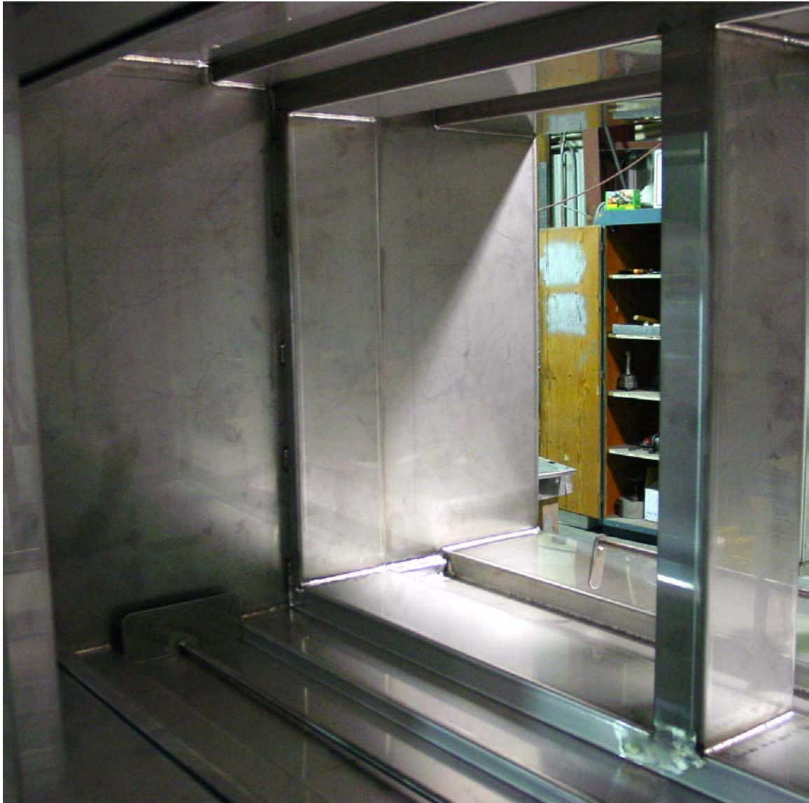
1H X 1W HEPA section- flat mounting surface Figure 1-4
