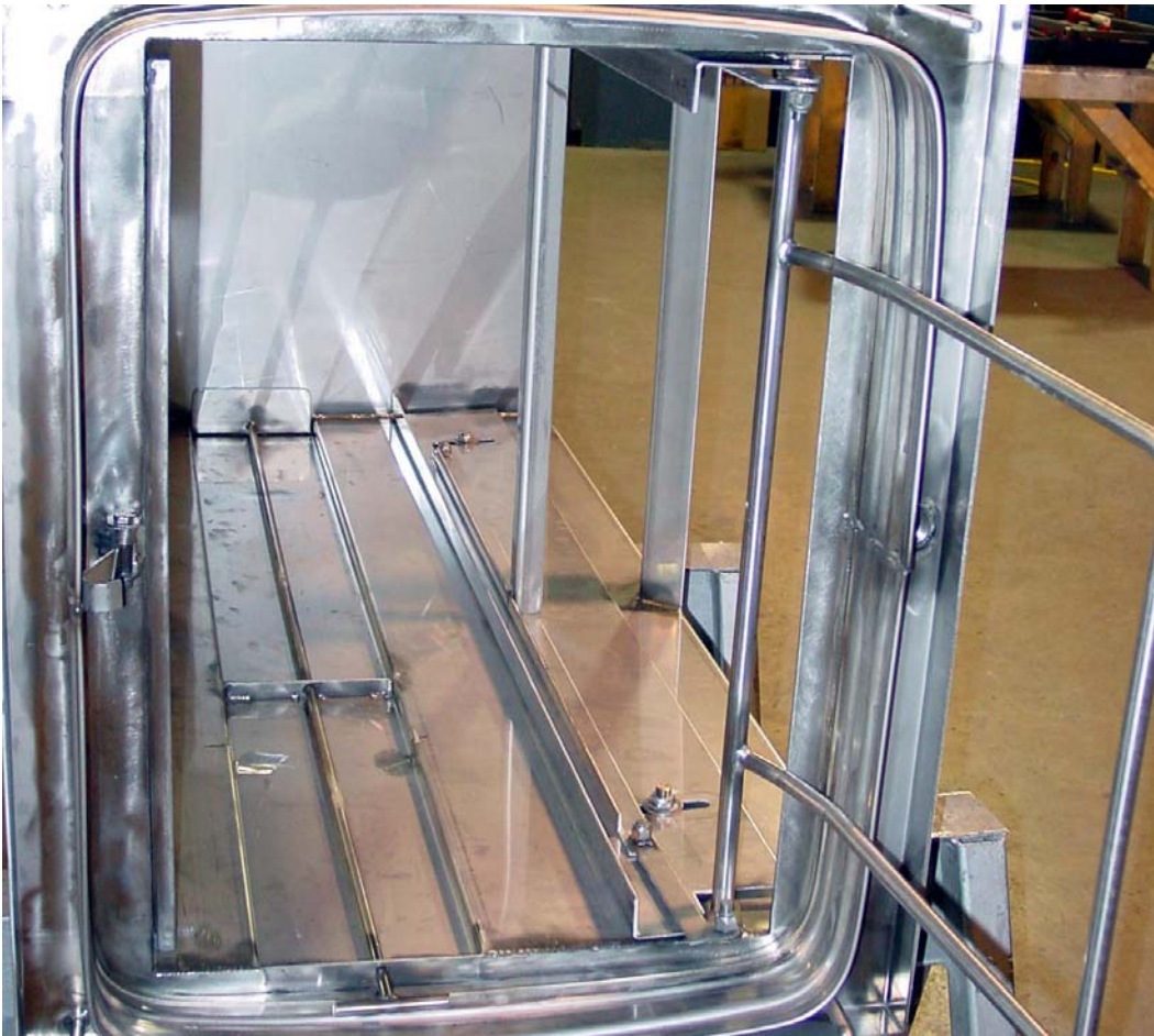
Locking arm of gel seal housing Figure 1-2
