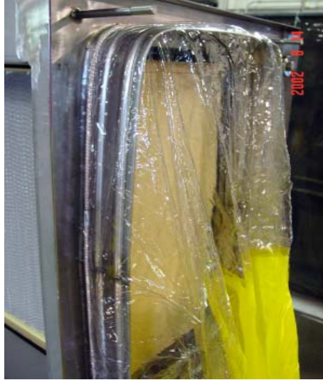
Note elastic bag strap is placed inside second rib Figure 1-9
