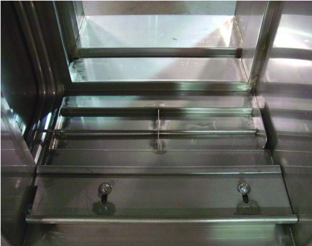
Downstream view of locking tray mechanism Figure 1-21
